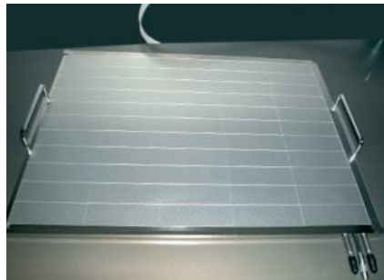
Exchangeable slide tray, suitable for refrigeration and designed to allow fixation of dispense targets*
