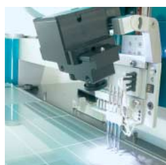
Observation camera, featuring two different magnification levels for manual teaching of XYZ positions.
